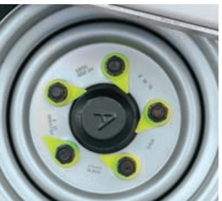
Wheel nut indicators out of alignment
