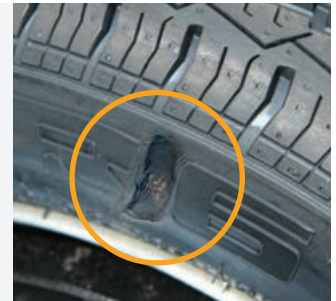
Damaged side wall
