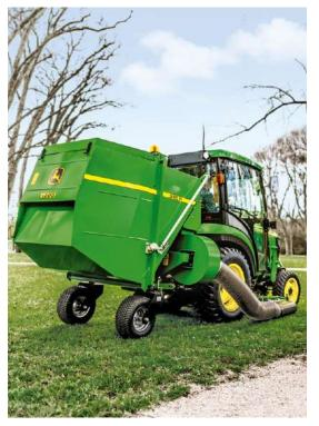
**580 L/H Collector:** The 600 or 850 litre collector has optional high dumping and one-handed hydraulic operation for easy unloading.
