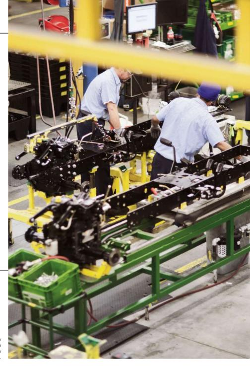
A transmission is being mounted onto the high-strength steel frame of a Compact Tractor by two Augusta factory workers.
