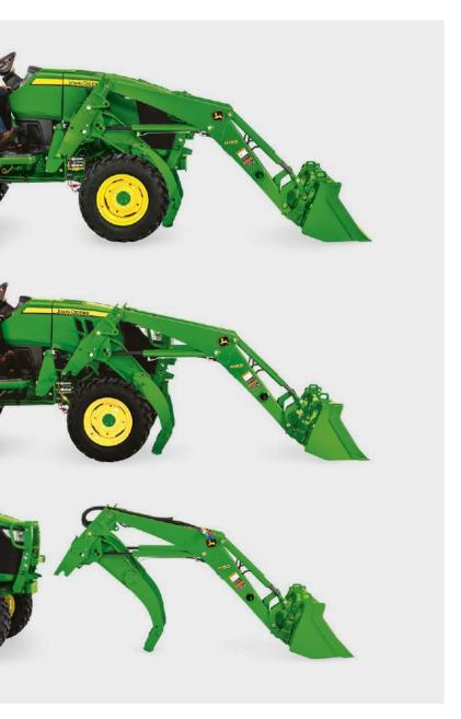
**Quik-Park loader mounting system:** H and R series loaders are designed for easy, tool-free mounting and removal. The parking stand is attached to the front frame of the tractor and becomes an integral part of the loader during loader operation. To drop the loader to the 'park' position, just lift the joystick after opening the latches.
