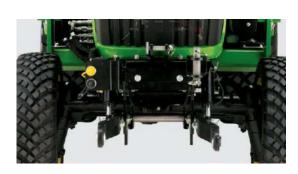
**Lift and Towing Hitches:** A wide range of efficient and powerful lift and towing hitches for both the front and rear, increase the versatility of your tractor.
