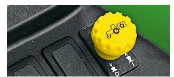
**Independent PTO**: Forget the days of stopping the tractor and manually engaging the PTO. With the electro-hydraulic PTO you can turn on your implement while you're on-the-go, so you can get your work done more quickly and easily.
